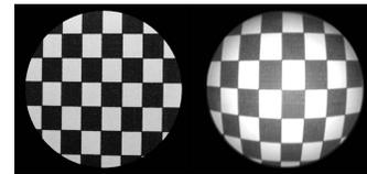
Figure 1. Chess pattern created (left) and the pattern acquired by endoscope system (right)
