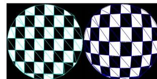
Figure 3. Mesh in the chess pattern image (left) and the mesh in the pattern image acquired by endoscope system (right)
