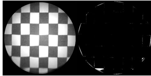
Figure 4. Result of application of the distorted image of chess (left) and the binary subtraction: distorted image processed minus chess pattern (right) using linear equations
