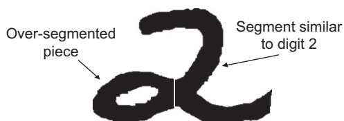
Fig. 10. Over-segmented "2" where the biggest segment can be easily confused with the digit "2".
